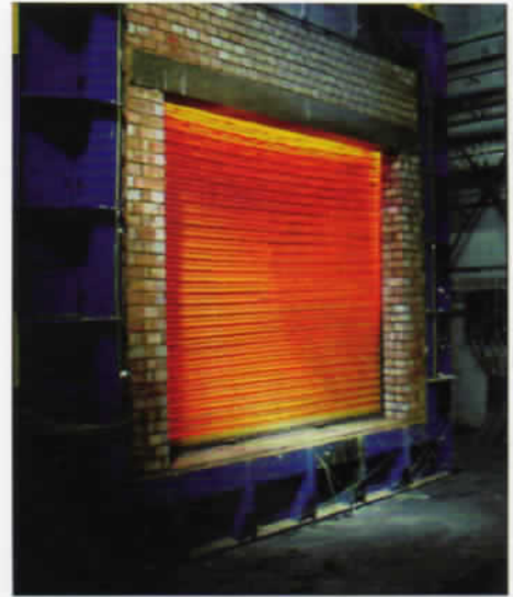
Shutter after 2 hours test
